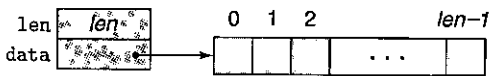
Figure 5.3 Vector abstract data type. A vector is represented by header information plus an array of designated length.
